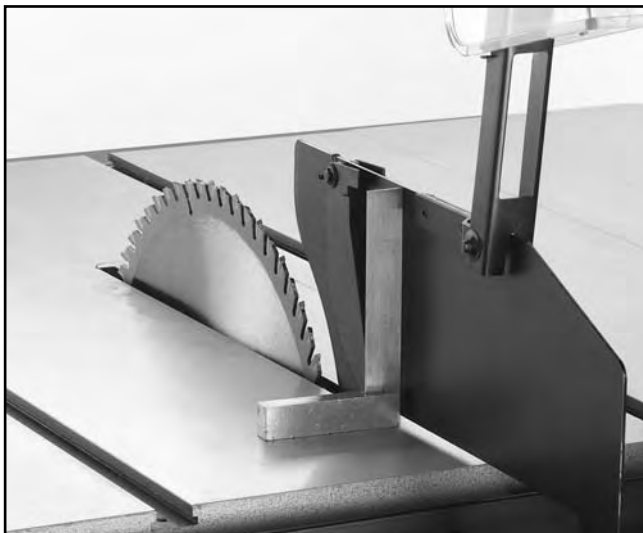
Figure 13. Guard assembly square to table.
